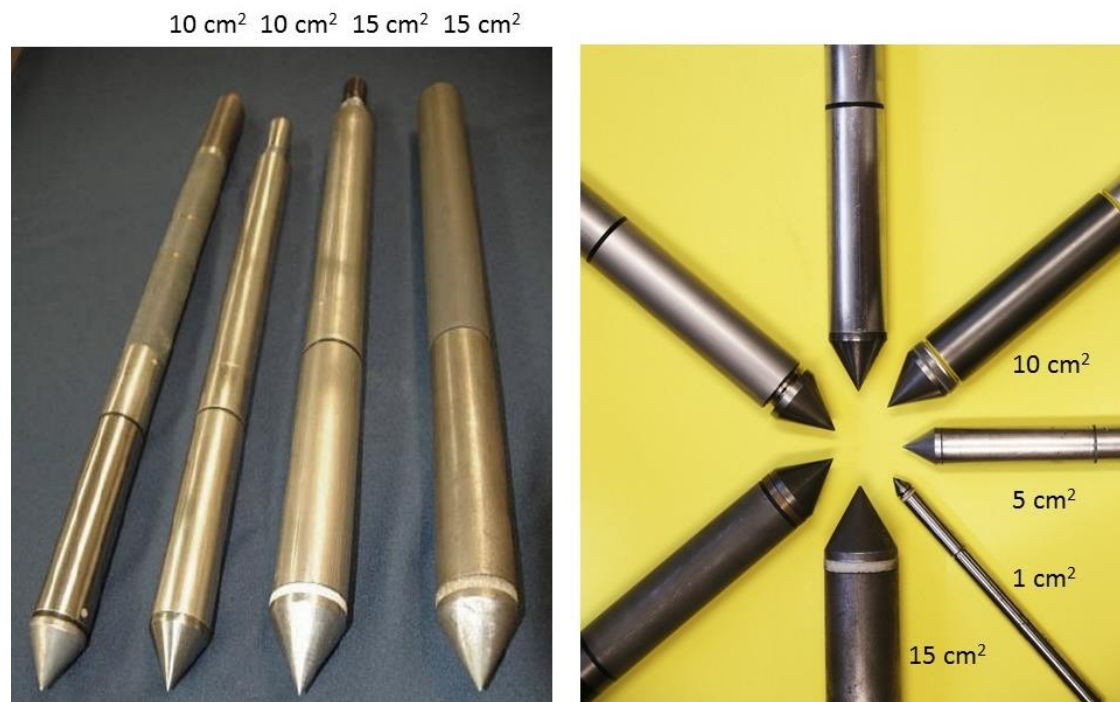
Figure 1.2: Family of Cone Penetrometers including: (a) standard 10- and 15-cm 2 sizes; (b) standard sizes in comparison with smaller versions
