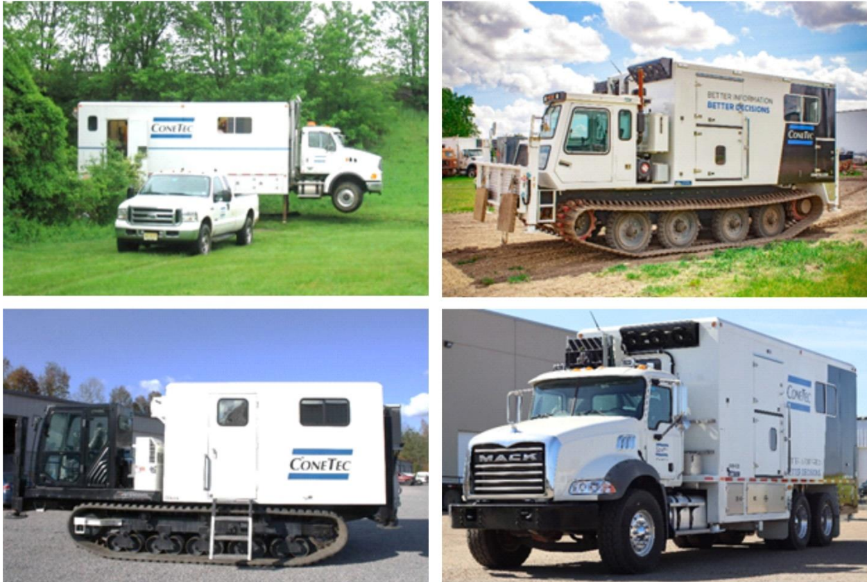
Figure 1.4: Various Truck- and Track-Mounted CPT Vehicles for Production In-Situ Testing
