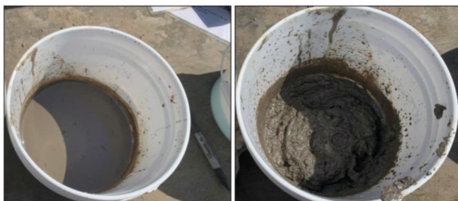
Figure 4. A segregated sandy sample before (left) and after (right) homogenization with sand suspending polymer.
